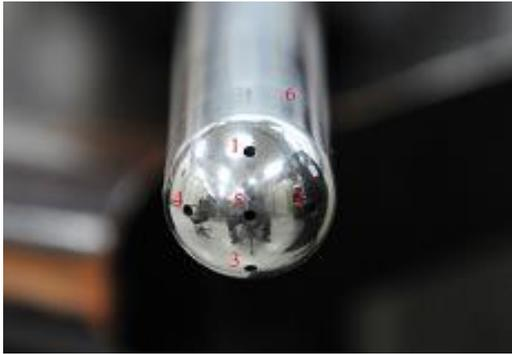
Gambar 3 Five-Hole Probe (FHP)
