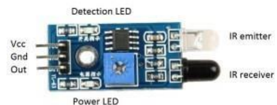
Gambar 8. Sensor Infrared FC-51
